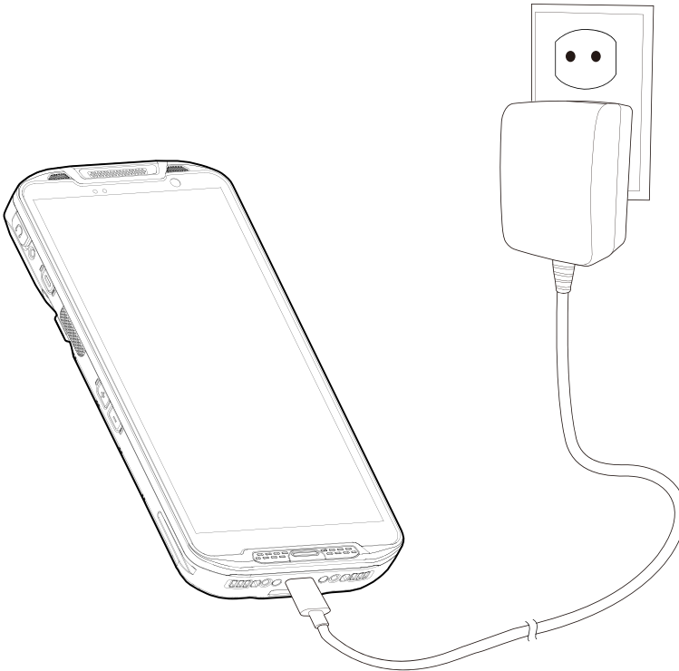
Figure 26 PM95 charging with power adapter
