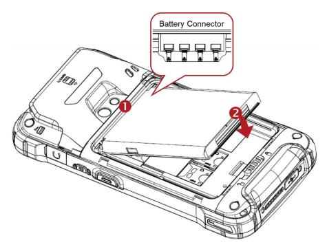
2. Insert the Battery Cover from the top area first and then put in bottom area. Press Battery Cover with both hand and Make sure **Battery Cover Lock** is **Lock** position
